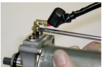
SECURE THE WIRE TO THE STARTER BY MEANS OF A PLASTIC CLAMP
